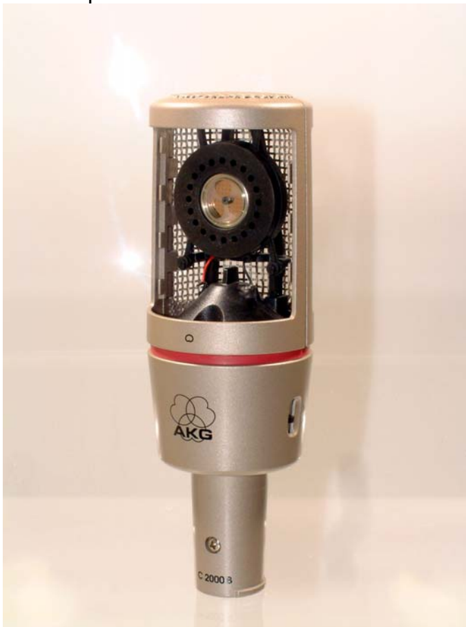
Fig. 1: Inside view of the AKG C 2000 B.
