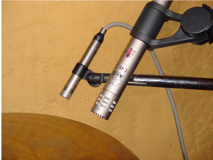
Fig. 1: Hi-hat with AKG C 451 B and reference microphone.
